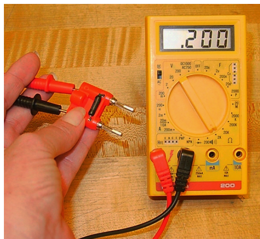
Fig. C-11: Ohmmeter and Resistor Ohmmeter Reading: 0.200\text{ k}\Omega=200\ \Omega .
