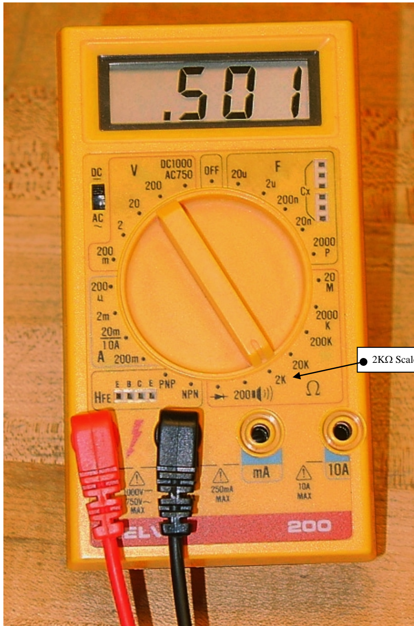
Fig. C-9: Ohmmeter Ohmmeter Reading: 0.501 \times 10^3 \Omega = 501 \Omega .
