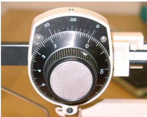
Fig. C-5 Dial zero aligns with vernier zero.
